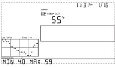
Values for the each of the last "MIN. 90. MHX. 59. 24 hours are displayed in the graph, each hour represented by a dot. The dot at right end of the graph is the value for the current hour. You'll notice that the dot is blinking.
