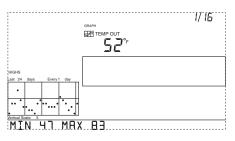
By pressing the down arrow again, the graph shifts to show the highs of the last 24 months. As before, use the right and left arrows to move between months. Press HI/LOW to shift between the highs and lows.
