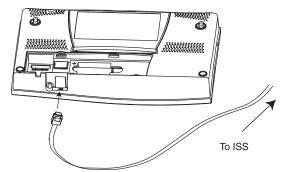
2. Ensure that the ISS cable is not twisted through the access port.
