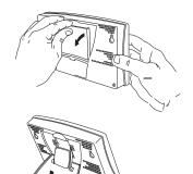
4. Install the two rubber channel feet on the kickstand.
